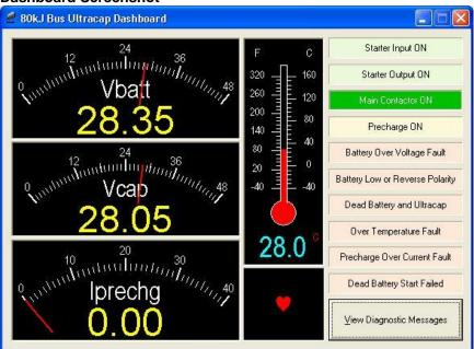
The left portion of the dashboard displays the battery and UltraCap voltages in addition to the Pre-charge current. The right portion of the dashboard illustrates status and fault messages.
