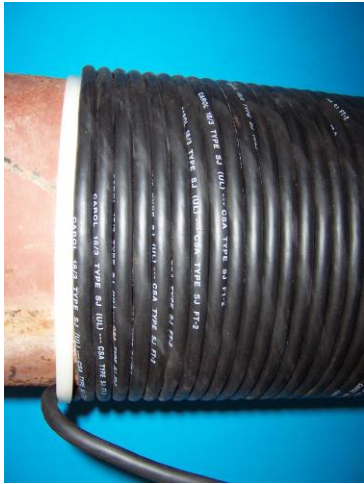
Photo 4a & 4b - Examples of tightly wrapped signal wire
