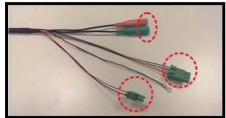
In addition, attach the ground cable to the ground and wrap the wires with silicone gel. Make sure the wires are not exposed to the air.
