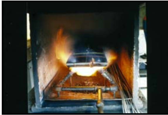
Test apparatus used to determine if conveyor belting meets the fire-resistance standards of BS3289
