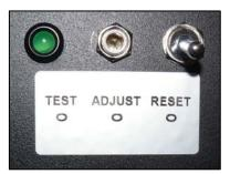
**RESET:** The new left-side control panel has three items. The toggle switch (reset) is a momentary closing switch, that has the same function as the reset button on the counter, but is more convenient for the operator.
