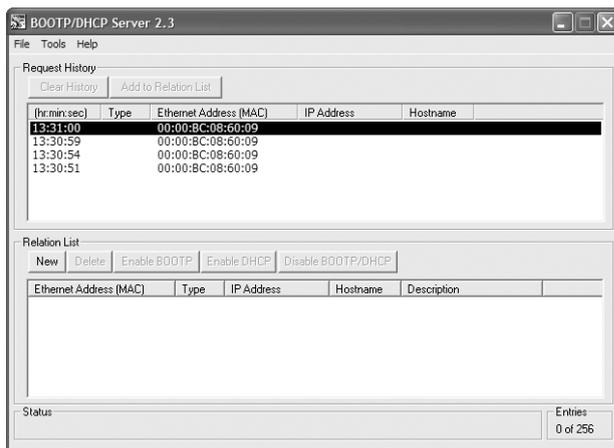
3. To properly configure devices on your Modbus/TCP network, you must configure settings in the BOOTP software to match the network. Select **Tools > Network Settings** to display the Network Settings window ([Figure 3.3](#)).
