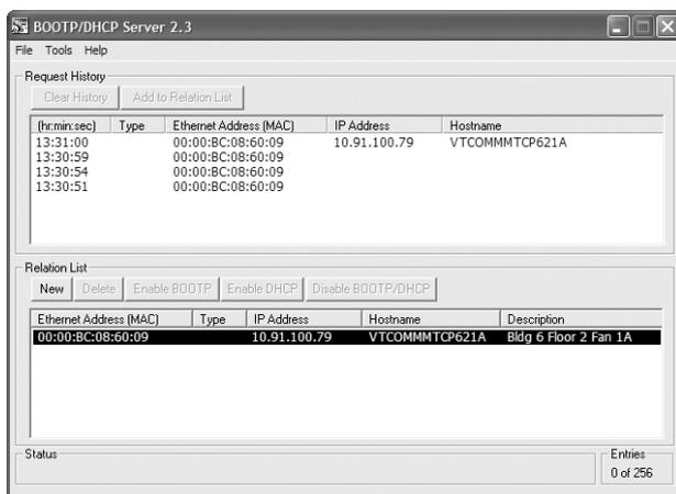
9. To assign this configuration to the module permanently, select the device in the Relation List and click **Disable BOOTP/DHCP**. When power is cycled on the module, it will use the configuration you assigned it and not issue new BOOTP requests.
