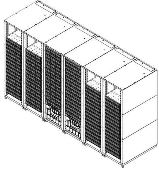
The XP7 hardware consists of one or two DKC racks that will hold up to 2 media form factor chassis in each DKC rack. There are three separate media chassis for 3 media form factors. Each media chassis may contain a maximum of
