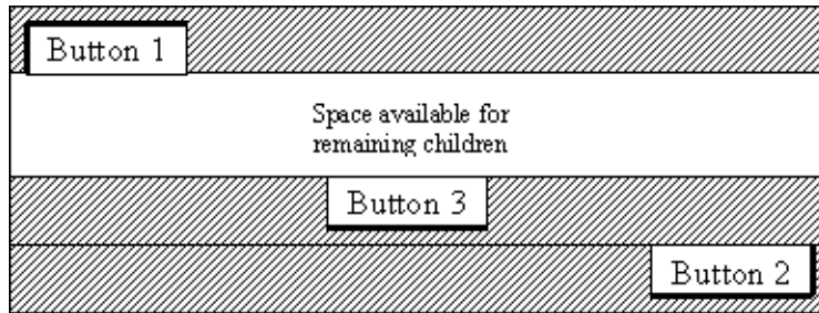
Figure 4–14 Adding a third button in the center at the bottom of the layout cavity.
