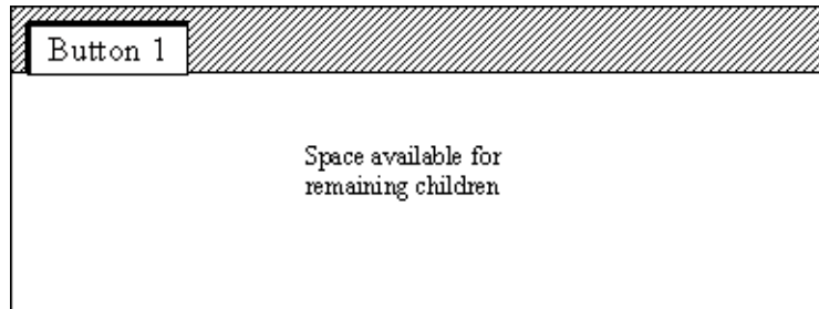
Figure 4–12 Creating a button on the left side and at the top of the layout cavity.
