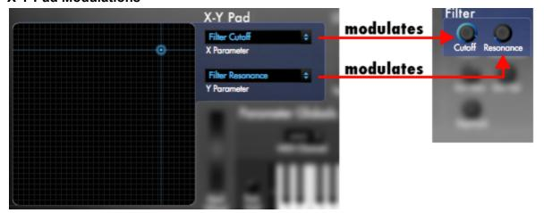
An obvious limitation of a knob on a computer GUI is that you can only rotate one knob at a time as you only have one mouse pointer! X-Y Pad Modulator works around this to allow you to control two paramters at once with the mouse.
