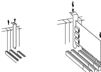
Remove the Slot Bracket
