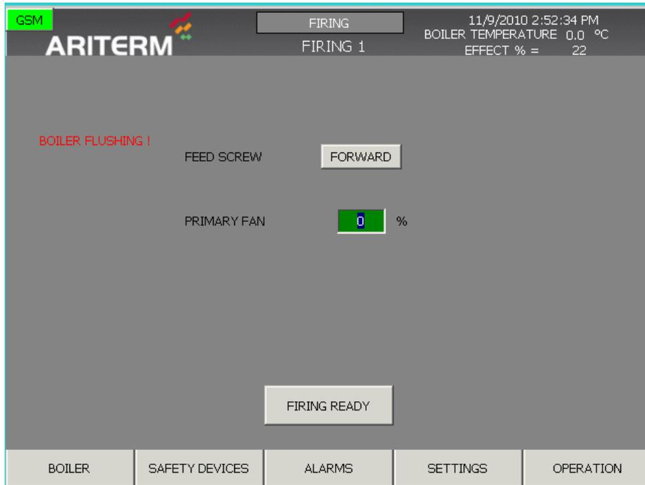
The burner is operated with a fixed power step which the user increases at his or her discretion. At this stage the user does not need to change the blowing strength, because the blowing percentages are determined by the set values in the power table, i.e. each power step has a certain control value for the fans.
