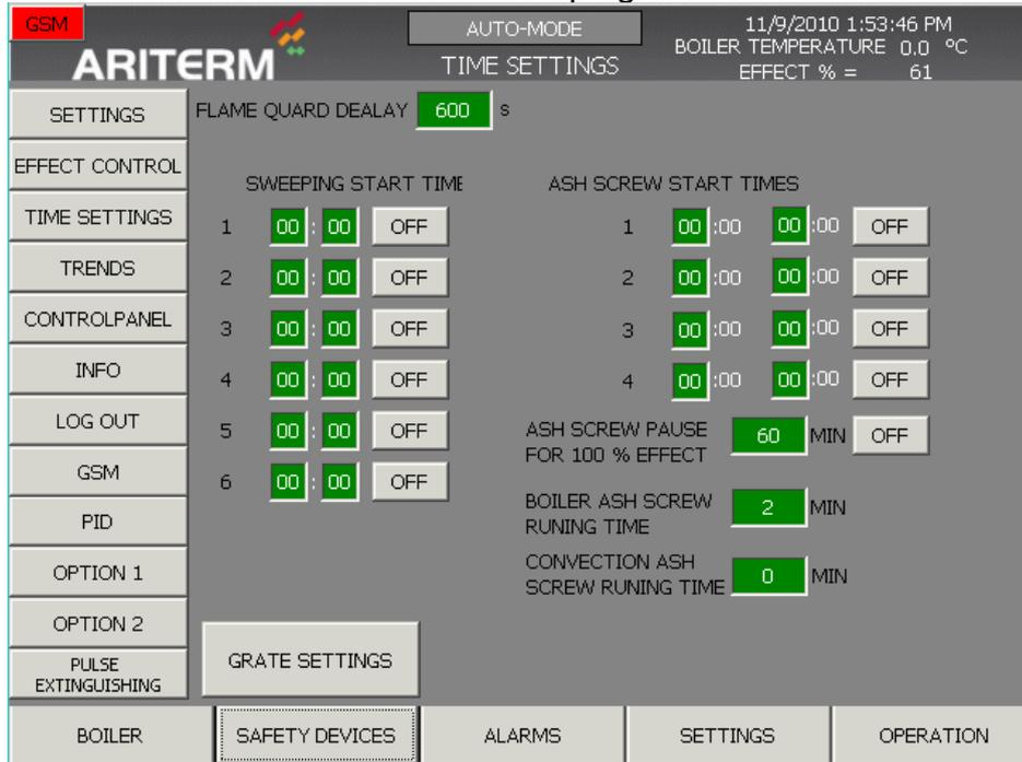
**Sweeping start times:** You can determine six times for the sweeping frequencies. The set time is activated with the ON/OFF button on the right side of the frequency field.
