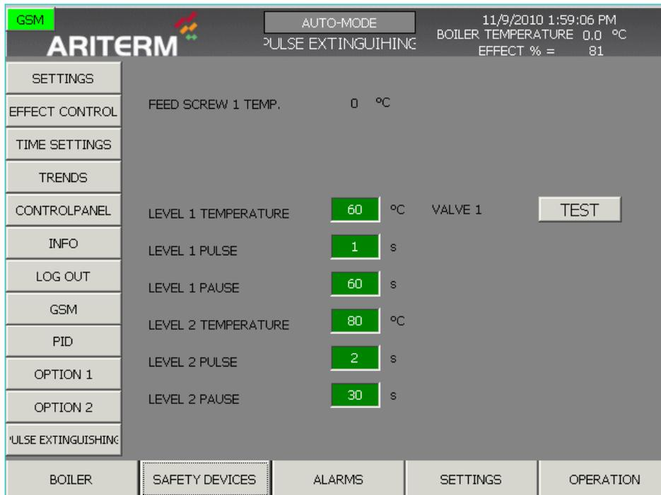
The pulse extinguishing system is used to prevent a back fire starting by dampening the fuel with water when the screw's surface temperature increases. The value "FEEDING UNIT 1 TEMPERATURE" indicates the current temperature on the screw surface. The surface temperature is measured using the PT100 sensor (4...20mA measuring message). There are two operational temperatures for dampening.
