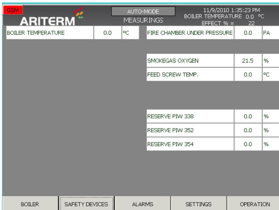
All the establishment's measurement values are on the Measurements page.
