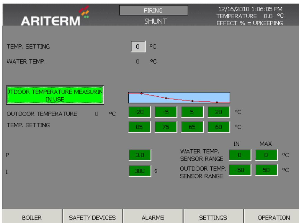
You can change the water control valve settings on the Shunt page. When outdoor temperature measurement is in use, the control valve adjusts the water temperature according to the outdoor temperature, as shown with the diagram.
