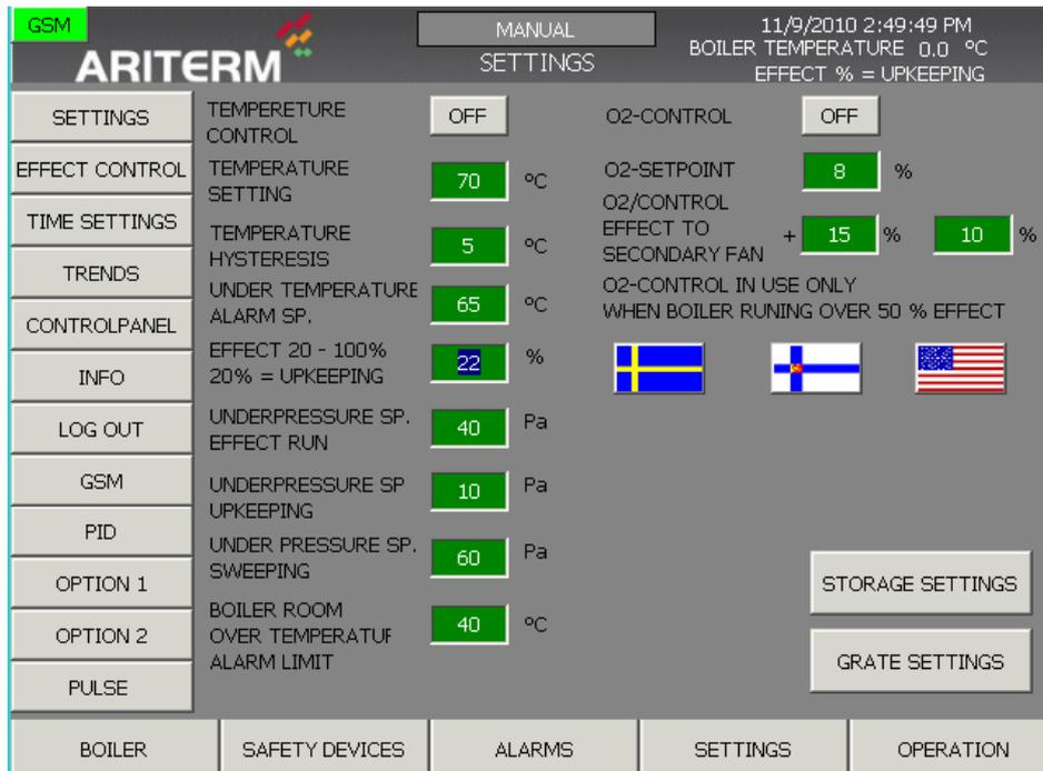
**"Temperature control"**: Select ON when you want the burner's power to be adjusted according to the power requirements.
