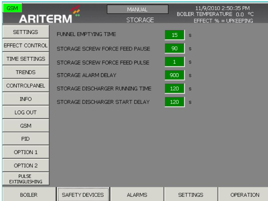
Storage screw 1 hopper emptying time: The hopper's lower limit is determined according to the feeding unit functioning time. When this theoretical time limit is reached, the storage screw is used until the hopper sensor indicates the upper limit.
