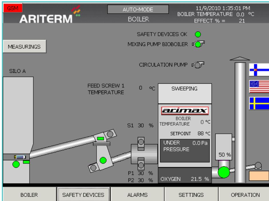
The operating panel "BOILER" page displays the following:
