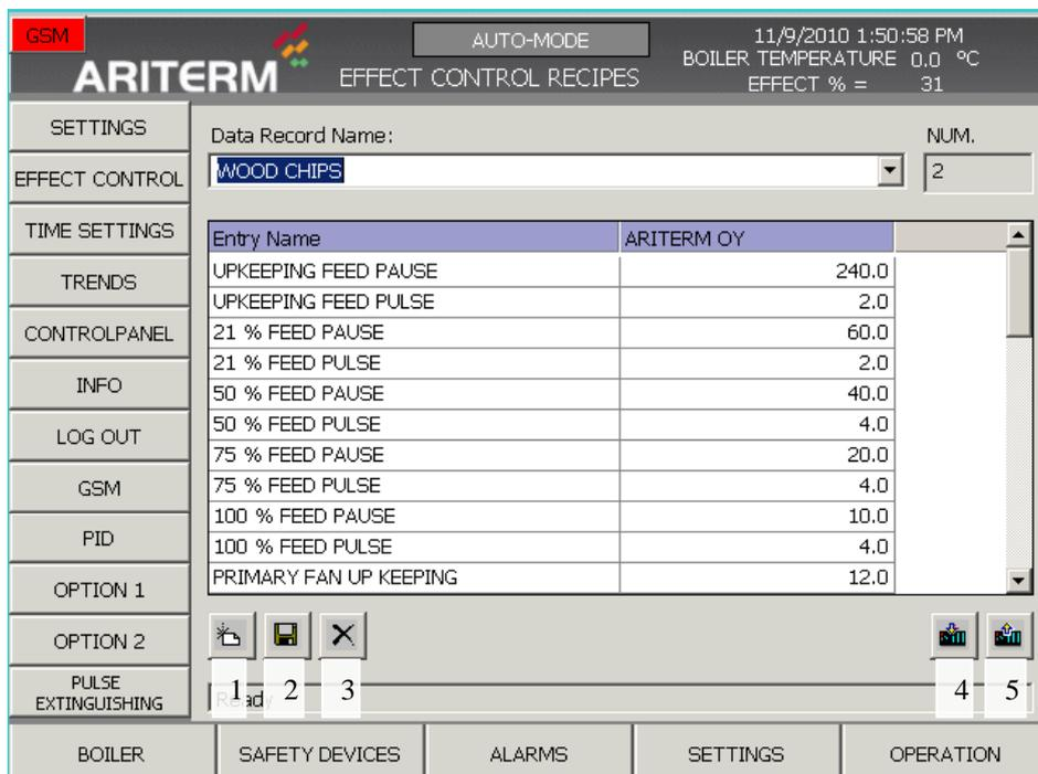
When you wish to create a new power table, press the number 1 button and determine the required **"Record name"**. When you have entered the required values in the fields, save them using the save icon (no. 2). The cross (no. 3) deletes the selected record.
