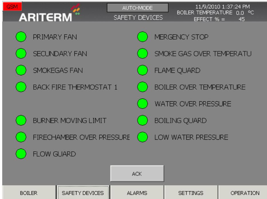
The "SAFETY DEVICES" page displays the status of the safety devices and alerts connected to the control computer. Active alerts are shown in red.
