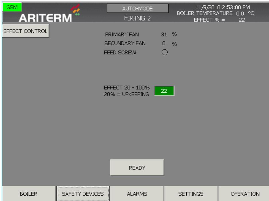
When the flue gas sensor detects the flame, the **"READY"** button turns green. When it is pressed the burner moves to automatic operation. The user does not need to wait for the flame information; he/she can press the **"READY"** button before this.
