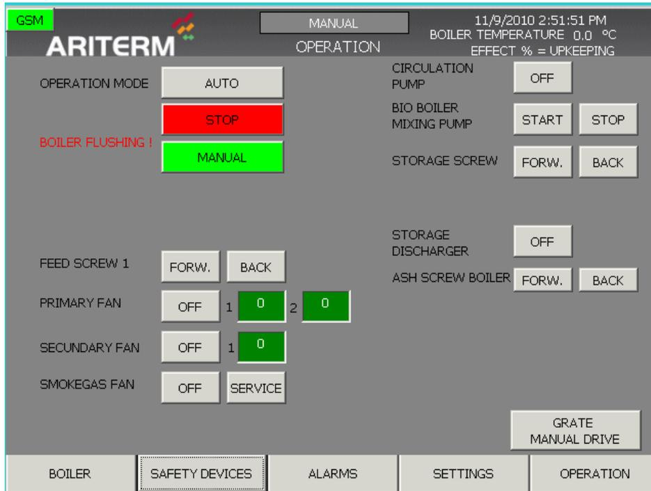
The "OPERATION" page is used to select how the system is operated. "AUTO" is the normal operating mode, when the system operates according to set operating parameters. When the "AUTO" mode is on, the "OPERATING" page can be used to stop/start the burner's cooling pump and the water's mixer pump. It is also possible to start pressure sweeping manually.
