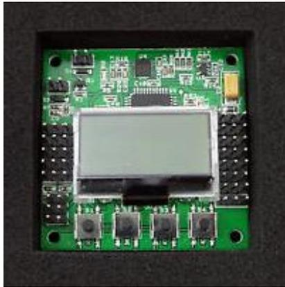
**STEP-1** Mount the FC on the frame with the LCD facing front and the buttons facing back. You can use the supplied anti-static foam container as a form of protective case for the Flight Controller on the craft.
