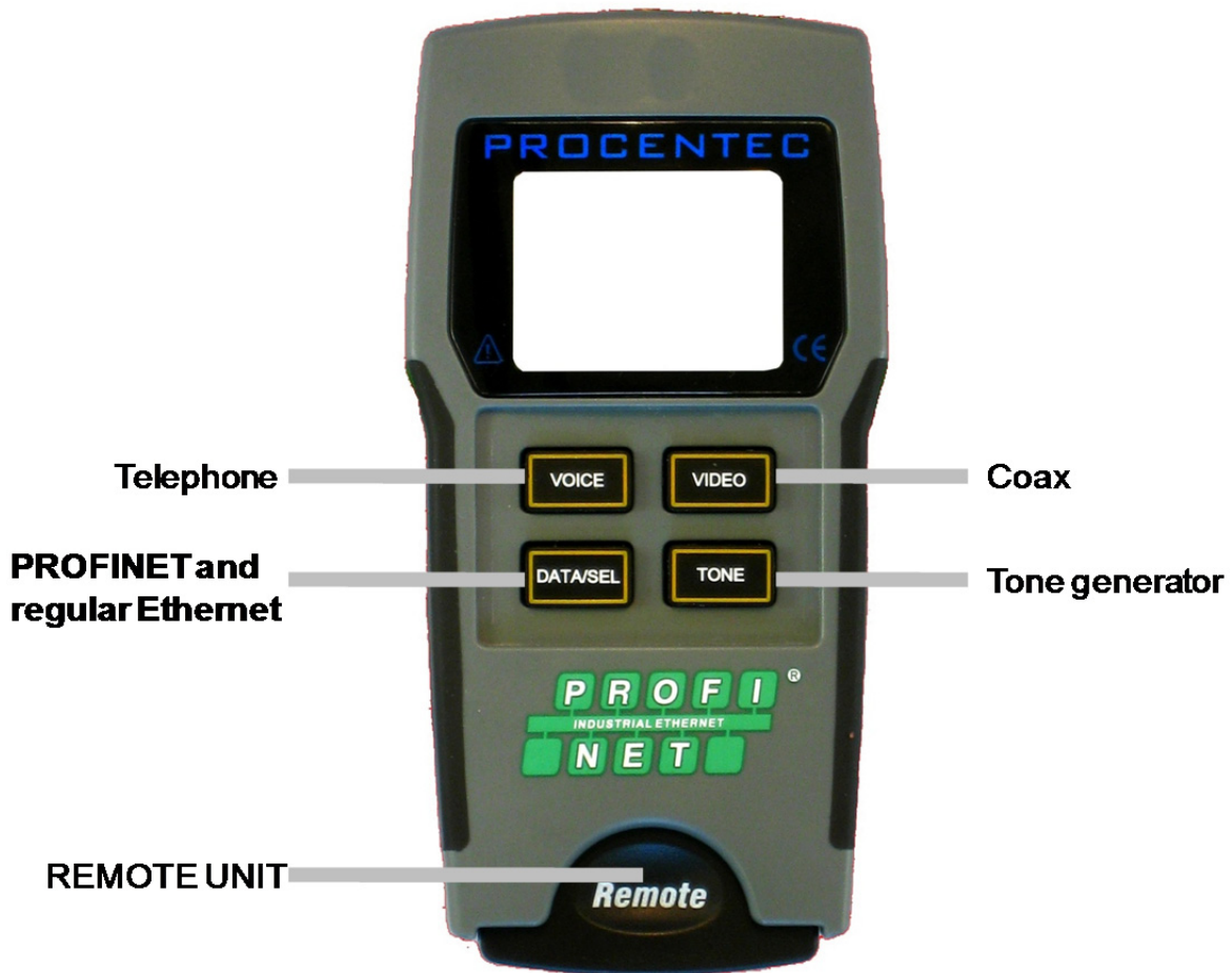
Fig. 1 - Location of the buttons and Remote Unit
