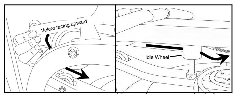
2. Next, thread the Belt around the Idle Wheel as shown. Once around the Idle Wheel, attach the Rower Belt to the Belt/Bungee Pulley. There is an obvious "lip" at the attachment point.
