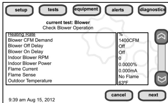
Figure 19. Typical tests results screens
