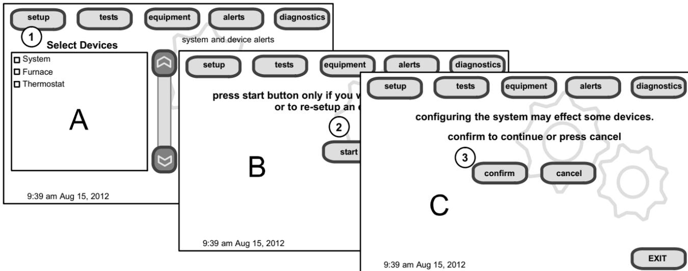
Figure 34. Re-configuration process
