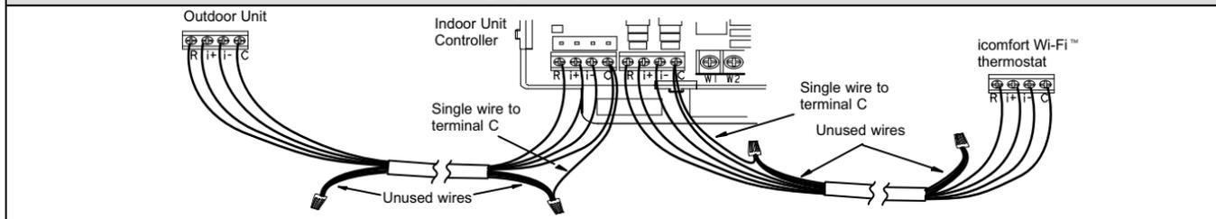
Communicating systems using the icomfort Wi-Fi™ thermostat require four thermostat wires between the thermostat and the furnace/air handler control and four wires between the outdoor unit and the furnace/air handler control. When a thermostat cable with more than four wires is used, the extra wires must be properly connected to avoid electrical noise. The wires must not be left disconnected.
