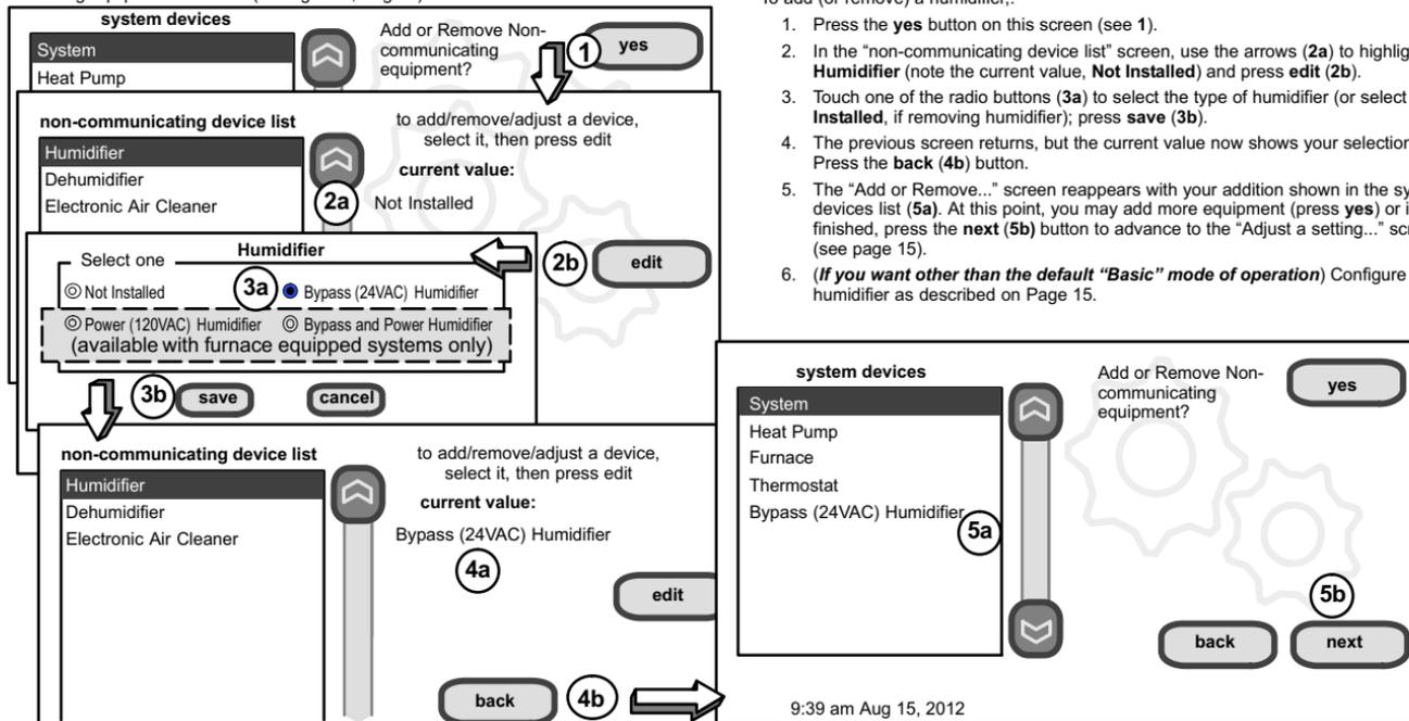
Figure 9. Add or remove non-communicating device—HUMIDIFIER
