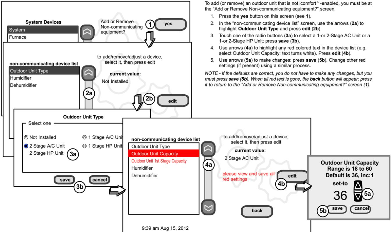
To add (or remove) an outdoor unit that is not icomfort™-enabled, you must be at the "Add or Remove Non-communicating equipment?" screen.
