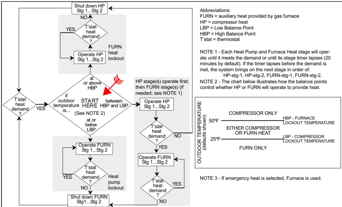
Figure 35. Dual Fuel Operation with Balance Points
