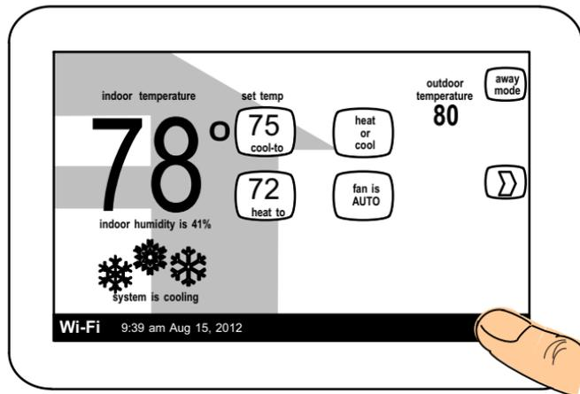
Figure 32. Enter installation setup mode from home screen
