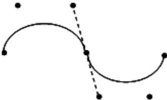
Figure 2.4 - A curve comprised of smaller Bezier curves
