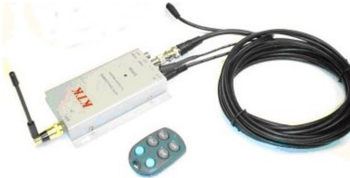
Recording Setup: Video receiver connected to the Trekker MiniDVR video input with manual KeyFob trigger
