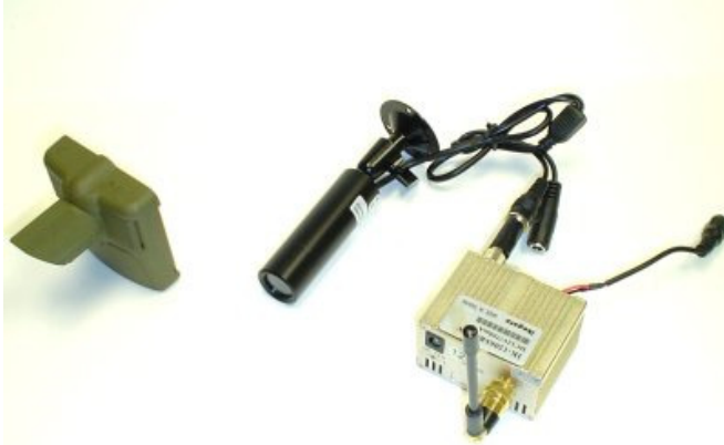
Room setup: PIR Motion sensor trigger, video camera connected to a wireless transmitter
