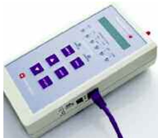
ParticleScan with network cable for direct connection to the network.
