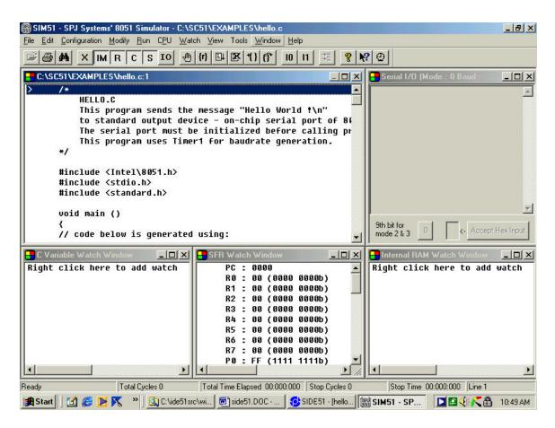
Please note that the program window is already open. In our example, the program simply sends a message "Hello World !\n" to the serial port. In order to debug the program, we must monitor the serial port output. It can be monitored in the Serial Port Window – which is already visible. To view / hide the Serial Port Window, select View/Serial window from the menu.
