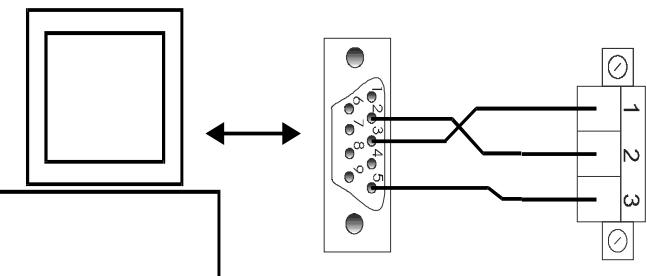
Use 9 pin DSub connector and connect with CON4 of the MC150 readout.
