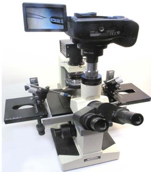
IMS-02 WITH MICROMANIPULATORS AND PIPETTE HOLDER AND DIGITAL CAMERA
