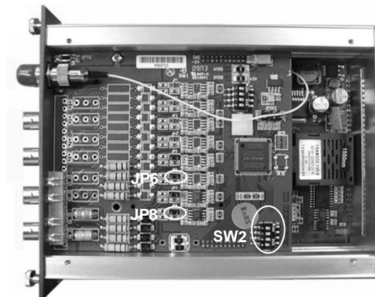
Figure 7. Location of on-board DIP switch
