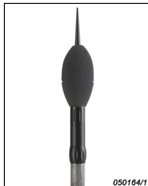
Fig. 2 Outdoor Microphone Type 4952 with integrated coupling, fitted on the top of a waterpipe
