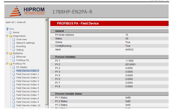
The web interface can be accessed by entering http:// IP address into the address bar of the browser as shown below:
