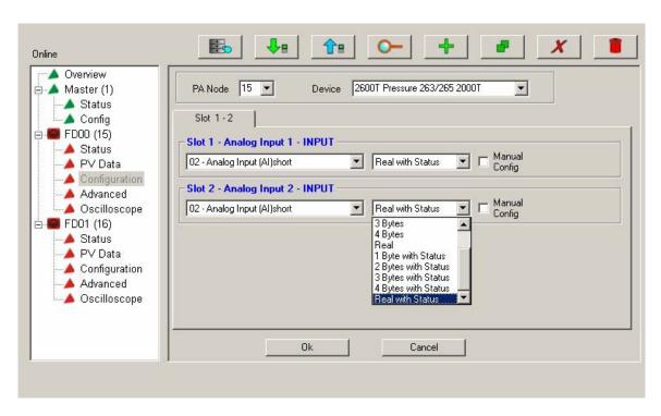
In some cases (eg. Positioner field devices) there are multiple input and output PVs per slot. The user will then manually need to configure the format for the slot. This is done be selecting the *Manual Config* tick box and clicking the configure button as shown below:
