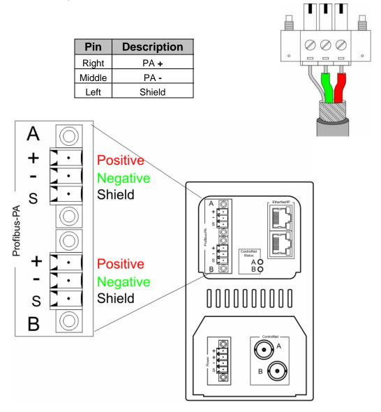
The PA cable color code is used as set in IEC61158-2 Physical Layer Specification.
