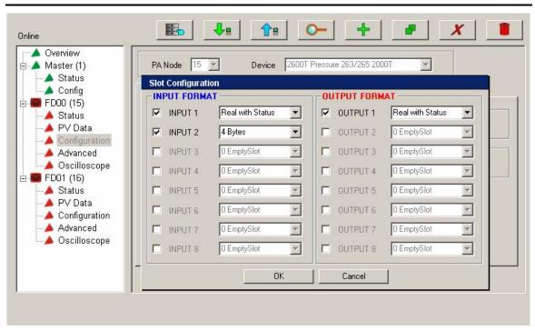
The user must select the number of inputs and outputs and their respective formats as given in the user manual of the field devices. In the input image of the field device the PV will be set as given in the manual slot configuration.
