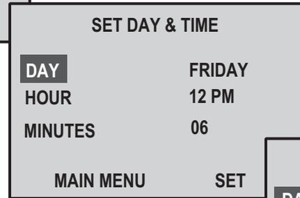
Use the UP or DOWN arrow to scroll through the days of the week, hours or minutes. Press SET to select desired value. Press MAIN MENU when complete.
