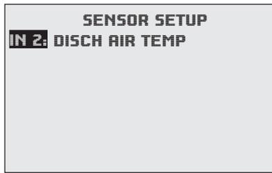
The Input 2 sensor (AI2) can be configured for discharge air temperature (Type III thermistor is the default), fan status (dry contact), or unused.
