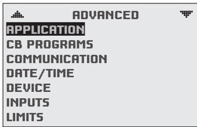
The Advanced Menu displays various submenus. Not all submenus can be seen on the screen at one time. Scroll up or down to see additional submenus. To select the desired submenu, press:
