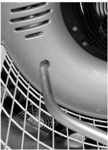
Slide the bottom of the handle into the lower handle bracket and insert a handle pin through it to lock the handle in place.
