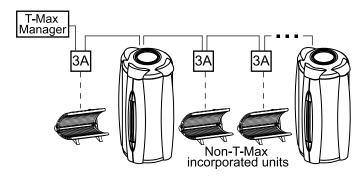
After you have set the T-Max® 1A's, or 3A's, address to "0" (refer to your T-Max® user's guide) and the booth's address to "1", simply connect the RJ-22 modular cables, described in the T-Max® user's guide, directly
