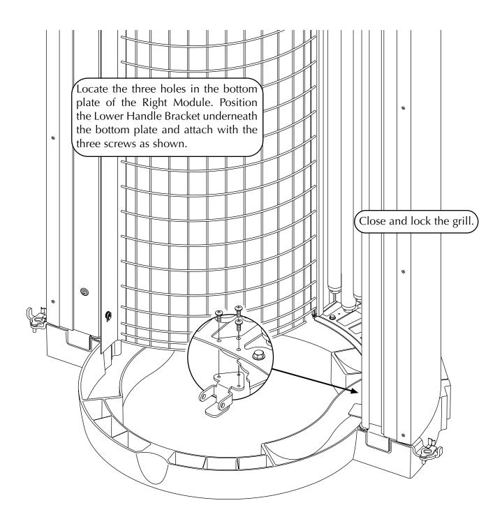
Parts needed: (1) Module Strap (2) #10 x 1" Phillips pan head screws
