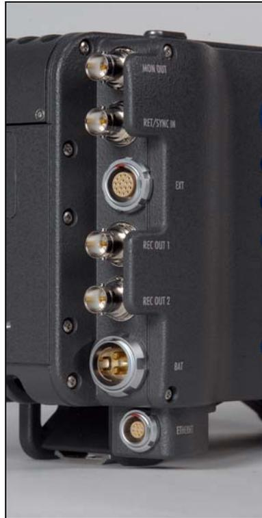
Figure 23: Connectors at back
