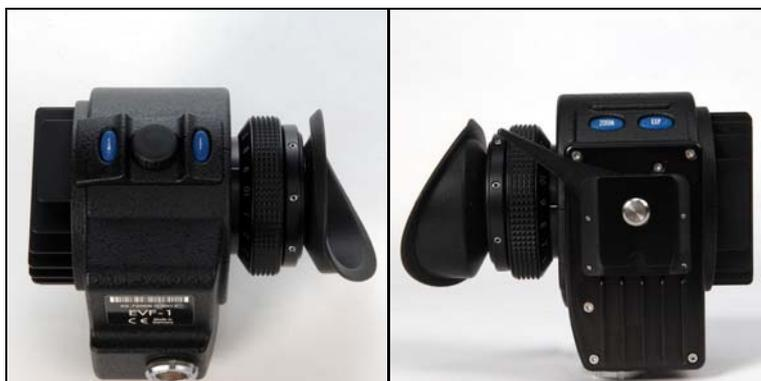
The EVF buttons are locked with the camera UI by pressing the LOCK button on the camera left or right side until the lock timer has elapsed. On the right side the timer is shown as a countdown on the display. The locked controls are visualized by a lock icon. On the left side the locked controls are visualized by a blue LED next to the LOCK button.
