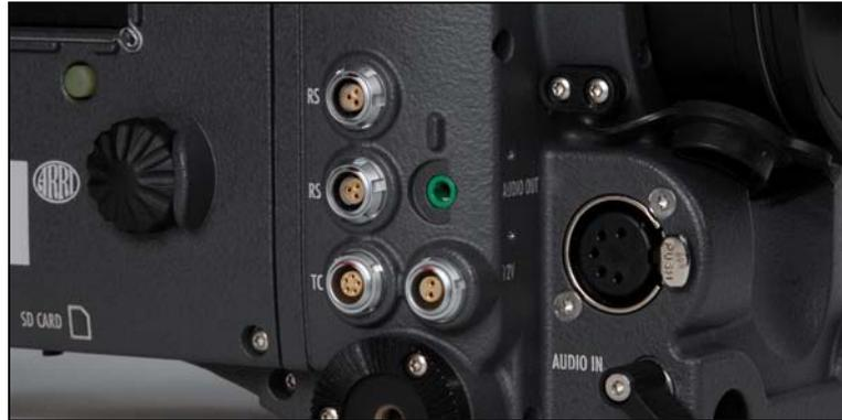
Figure 10: 24 V outputs (RS) and 12 V output
