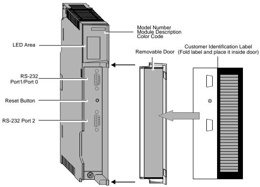
The ESI features two serial ports that can sustain communication rates of up to 9600 baud. Programming the ESI is done using port configurations and ASCII messages through one of the serial ports using a dumb terminal or with a personal computer using terminal emulation software. The ASCII messages are initiated by using logic running in the Quantum controller.
