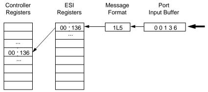
**Note:** Enusre the number of incoming characters match the number defined in the ASCII message. If in the above example the device sends "0013", the ESI module would not be able to finish the receive command and would wait until reception of a 5th character.
