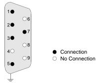
Pinout for the RS-232 ports:
