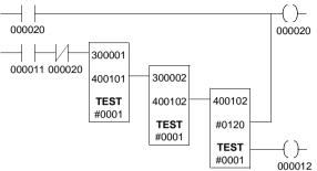
As long as coil 000011 is ON and coil 000020 is OFF, PUT DATA response word 0 in the input register is tested to make sure it is the same as the command word in the workspace. The module start register in the input register is also tested to make sure it is the same as the module start register in the workspace.
