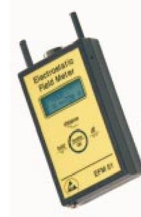
**Small hand-held Electrostatic Field Meter with digital display designed to measure electrostatic charges and fields according to the field mill induction principle.**
