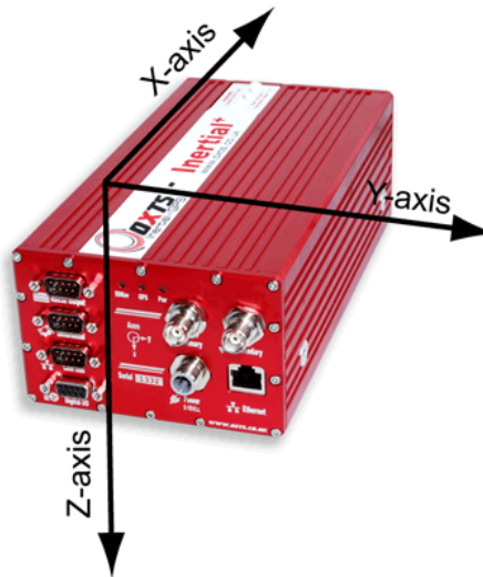
Figure 23. Inertial+ Co-ordinate Frame Definition
