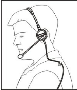
The headset consists of an earpiece, a microphone, a clothing clip and a cable. The headset attaches to the audio cable end of the voice cable which attaches to the MX8.
