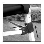
5. Engage auto-slider at each corner by pushing up on slider with one hand while pushing down on top of leg with other hand. Snap button will engage in hole. Repeat step on remaining legs.
