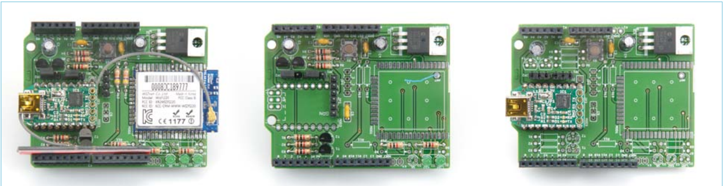
Figure 4. The three main configurations next to each other. The Bluetooth module is not visible (middle board) because it is mounted on the other side of the PCB. Note that this is an early revision of the PCB that has the same shape as an Arduino Uno board. The final PCB is rectangular.
