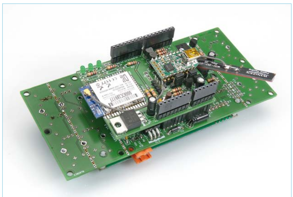
Figure 2. Fully built-up Wi-Fi shield on top of Platino, also equipped with a 20x4 alphanumeric LCD.
