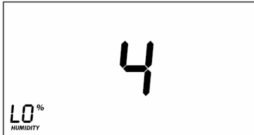
LCD display when using Up or Down arrows to select from the 4 controller groups.
