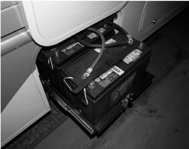
4. To store batteries, push slide tray in until it “clicks” into locked position.
