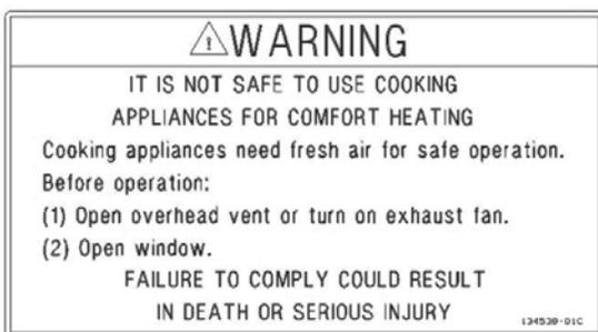
Unlike homes, the amount of oxygen supply is limited due to the size of the recreational vehicle, and proper ventilation when using the cooking appliance(s) avoids dangers of asphyxiation. It is especially important that cooking appliances not be used for comfort heating, as the danger of
