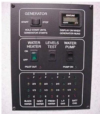
At the touch of a button this panel will display the fresh water and holding tank levels, propane gas tank level, plus the house battery condition. You can start the generator or turn on the water pump and water heater. Indicator lights tell you if the water pump is on or if the water heater pilot light is out.
