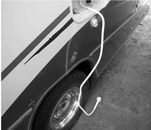
Using exterior shower to drain waterline (if equipped)
