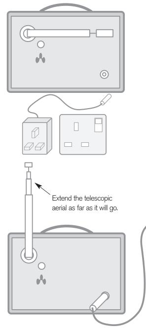
As soon as the power is connected to the radio it will automatically enter into auto tune mode.
