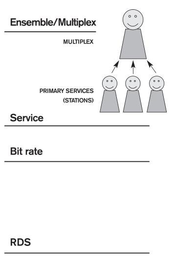
Stands for Digital Audio Broadcasting. Analogue radio is transmitted by placing the audio onto a carrier. If there is any interference or static with the wanted signal then it will be heard on the receiver's speaker. Digital however is transmitted in the form of a digital stream. The decoder in the radio knows what data is needed to re-construct the original signal, so any other unwanted signal is discarded.
