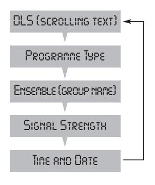
The information is displayed on the lower segment of the LCD display.
