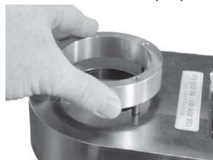
**Figure 14. Placing second spacer on roll pins**
