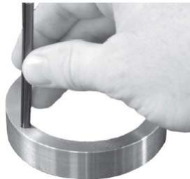
**Figure 12. Inserting roll pin**
