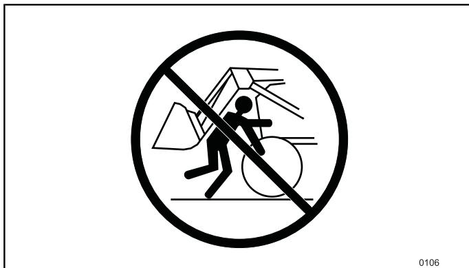
Fig.91 Never stand between the front of the tractor and the loader's cross tube.
