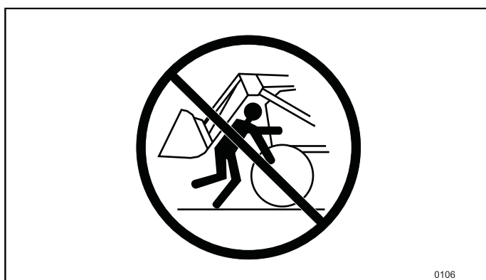
Fig.73 Do NOT stand, walk or work under a lifted loader.
