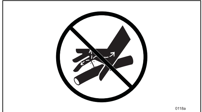
Fig.94 NEVER use fingers or hands for leakage detection.
