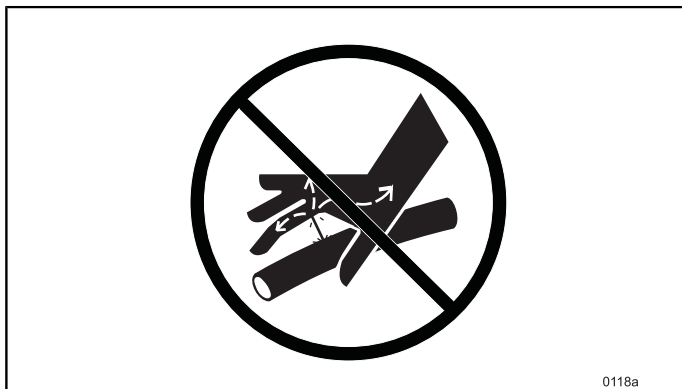
Fig.93 NEVER use fingers or hands for leakage detection.
