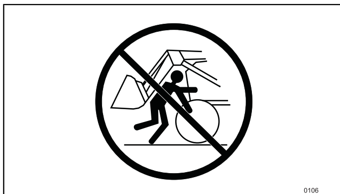
Fig.33 Never stand between the front of the tractor and the loader's cross tube.
