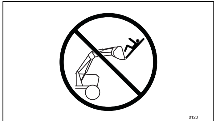
Fig.23 Do NOT use the loader or the bucket as a working platform.
