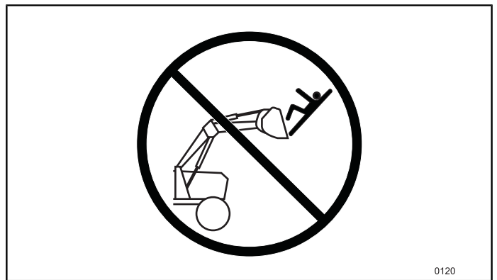
Fig.70 Do NOT use the loader or the bucket as a working platform.
