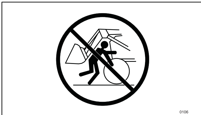
Fig.25 Do NOT stand, walk or work under a lifted loader.
