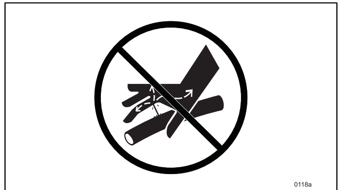
Fig.37 NEVER use fingers or hands for leakage detection.
