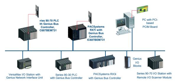
A bus may be used entirely for I/O control, or it may feature I/O control enhanced by communications commands in the program. A bus may also be dedicated to CPU communications, with multiple CPUs and no I/O devices. Communications can include transmitting Global Data from one CPU to another. The Global Data area is identified in the configuration. After initialization, the specified data area is transferred between devices automatically and repetitively.
