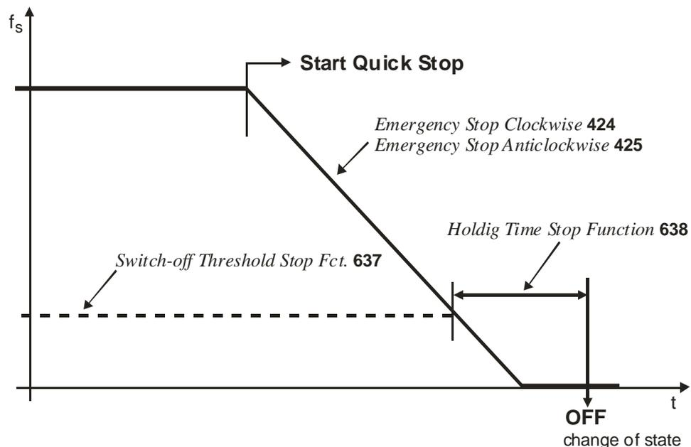
If frequency/speed reaches the value zero during the switch-off time, the drive continues to be supplied with current until the switch-off time has elapsed. This ensures that the drive is at a standstill when the state changes.
