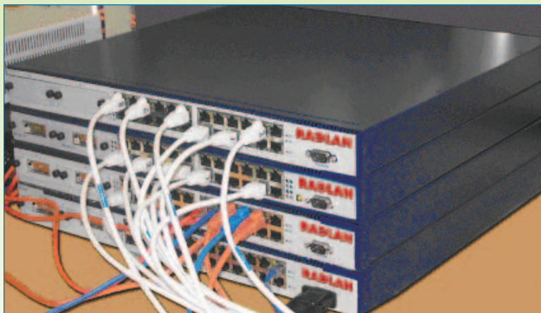
FIGURE 3: Stacking capabilities allow low-cost 'pizza box' switches to be combined to form a single larger unit.
