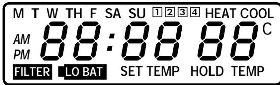
Display shows time, day, temperature, program number, hold, usage and low battery indicator.
