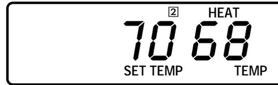
■ 70 indicates the current setting of the thermostat is 70°F. 68 shows the present room temperature as 68°F.
