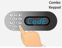
STEP 2: Sign "CodE" starts flashing beep acoustic signal is heard.
