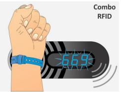
If the RFID media is presented and recognized as a locker key on different device the locker number is flashing on the display and interrupted acoustic signal is activated. Locker remains closed.
