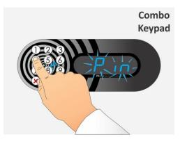
STEP 2: If PIN code was chosen sign "Pin" is flashing and beep acoustic signal is heard. Enter the PIN code that was used to lock multiple lockers and confirm it with  $\checkmark$  key.
