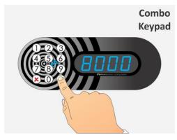
**STEP 1:** Enter group PIN code (number defined by "GrUP" parameter – from 8000 to 9999) to start multiple locking procedure and press the ✓ key.
