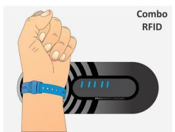
**STEP 2:** Approach the RFID media to the antenna field. Reading distance is 2 - 5 centimetres from the device surface. Hold the RFID media in the field for a few moments for device to read and process it.
