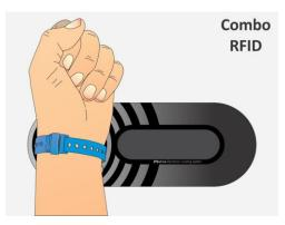
**STEP 1**: Approach the RFID media to the antenna field. Reading distance is 2 – 5 centimetres from the device surface. Hold the RFID media in the antenna field for a few moments for device to read and process it.
