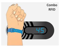
**STEP 2:** Display shows the locker number and the locker is unlocked when the RFID media is recognized as a locker key that previously locked that particular locker. Short acoustic signal is also activated.
