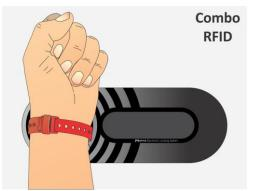
STEP 1: Approach the User / Multi key to the antenna field. Reading distance is 2 - 5 centimetres from the device surface. Hold the RFID media in the antenna field for a few moments for device to read and process it.
