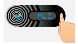
All the lockers connected to that Locker Controller start to unlock and open one after another and corresponding locker numbers are displayed.
