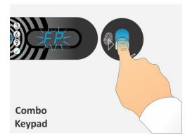
**NOTE:** If **fingerprint** was chosen sign "FP" is flashing and beep acoustic signal is heard. Insert your finger in the Fingerprint module.
