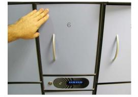
**STEP 1:** Close the locker door. Time countdown starts (vertical lines are displayed) on the Display and interrupted beep acoustic signal is activated.
