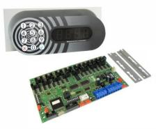
Metra Electronic Locking System (ELS) is primarily designed and used for locking lockers. Each ELS system has two basic components: Metra Locker Controller and Metra Display. Locker Controller drives and monitors up to 16 locks connected directly to the unit, with the possibility to add up to two Extension Modules for 8 additional Electronic Locks each. This enables configurations of 16, 24 or 32 locks, which makes the controller adoptable to many locker layout configurations.
