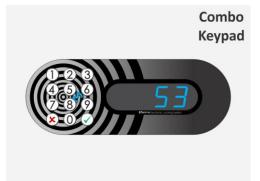
**STEP 4 A:** If "ALL" was confirmed corresponding lockers start to unlock and open one after another and corresponding locker numbers are displayed.
