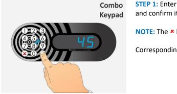
**STEP 1:** Enter the number of the locker you want to open and confirm it with  $\checkmark$  key.
