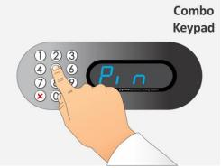
**STEP 2:** Sign "Pin" is flashing and beep acoustic signal is heard. Enter the PIN code that was used to lock corresponding locker and confirm it with ✓ key.
