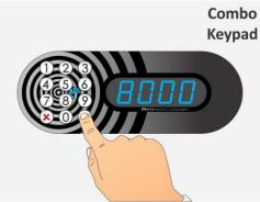
**STEP 1:** Enter group PIN code to start multiple unlocking procedure and press the  $\checkmark$  key.
