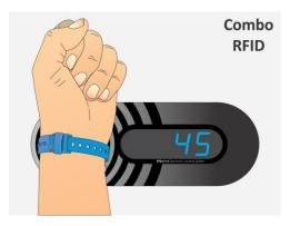
**STEP 3:** When the RFID media is accepted as a locker key the corresponding locker is locked and its number is displayed.
