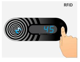
**STEP 1:** Select the desired locker number by pressing the 'up' key to increase or the 'down' key to decrease the currently selected locker number. Use the "Enter" key to confirm the unlocking of selected locker.
