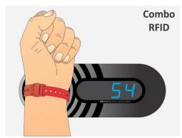
STEP 3 A: To open all lockers at once present the User / Multi key again to the antenna field when sign "ALL" is displayed.
