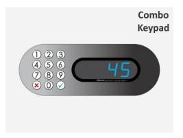
**STEP 3:** If correct PIN code is entered, locker number is displayed and corresponding locker is unlocked and opened. Short acoustic signal is also activated.
