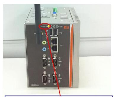
When the BIOS finish the configuration of system, the LED of ACT/RDY will ON.
