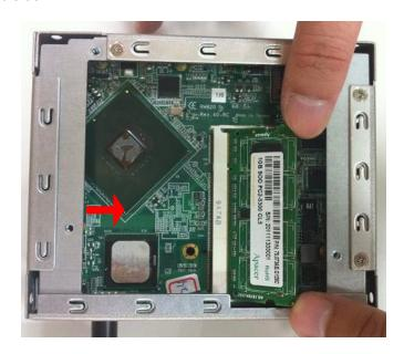
**Step 4** The memory module is locked by two latches on the sides.
