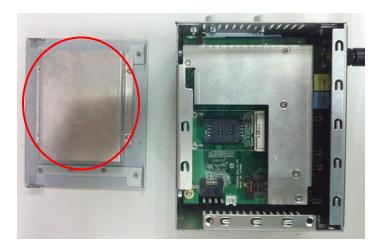
**Step 4** Loosen these screws and remove the Hard Disk Drive bracket.
