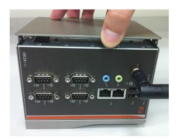
**Step 3** Locate the Hard Disk Drive socket.
