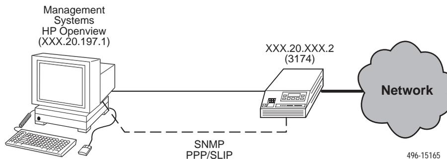
**Figure A-3. Connecting Devices Using a SLIP/PPP Connection**
