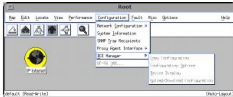
The remaining chapters in this manual describe how to use the DCE Manager with the OpenView user interface. Although the OpenView and NetView interface differ somewhat, the function of the DCE Manager is the same.
