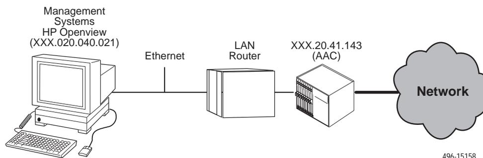
**Figure A-2. Connecting an AAC Device Using a LAN Router**
