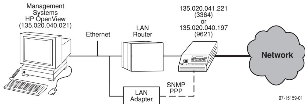
**Figure A-1. Connecting Devices Using a LAN Adapter**
