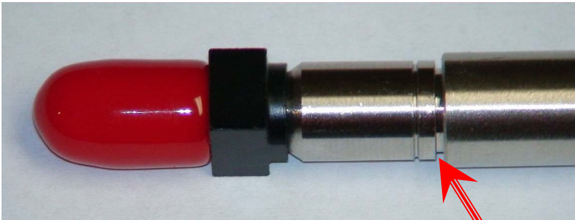
2 TSC-100F tip not fully screwed into the EXT-4 extension
