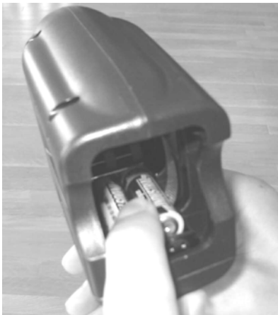
5 Once the positive pole is in place, push the battery down in final position.
