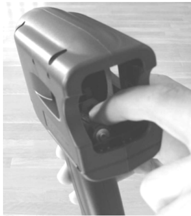
2 Once the negative pole is in place, push the battery down in final position.
