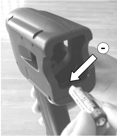
1 Install the first battery in the left position with positive pole outwards.
