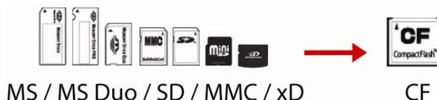
1. First, insert the card (MS, MS Duo, MS PRO Duo, SD, MMC, or xD) with the files you want to copy into the corresponding card slot. Photo Safe II will display the memory card type and amount of data on the card. The **{COPY}** icon will flash, indicating that Photo Safe II is ready to copy.
