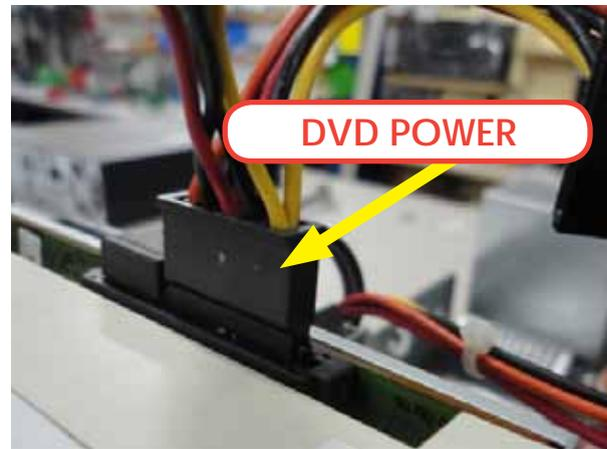
11. If all connections are fine (as it appears in the pictures), then it is possible that the component, which is not detected at the "IDE CONFIGURATION" Menu, is physically damaged. Please contact Digital Centre for a new part.
