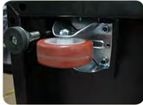
Adjust the height of the four metal legs once the final location for the booth has been established. The screws are underneath the cabin next to the wheels.
