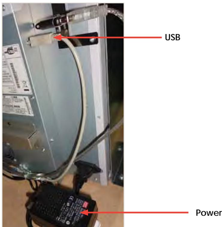
3- Check the Control Board Serial Connection. (That is the common problem Point). (attached 2 pictures: Correct and Error "Please Wait"). This connection is very easy to lose during transport, or when we work at that area.
