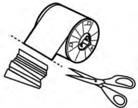
When the manual feed & cut mode has been selected, hold down the FEED & CUT button for 1 second or longer. Repeat the manual feed & cut three times. When the print paper with the postcard printing on its reverse side is installed, repeat this procedure five times.
