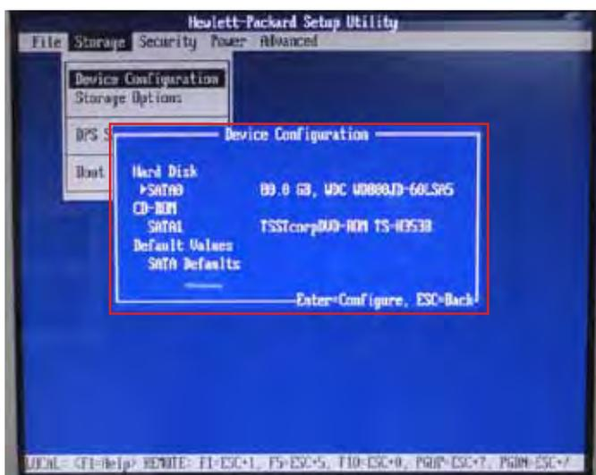
4. With the Keyboard arrows, move up to the Storage Menu, here we are going to check the following thing:
