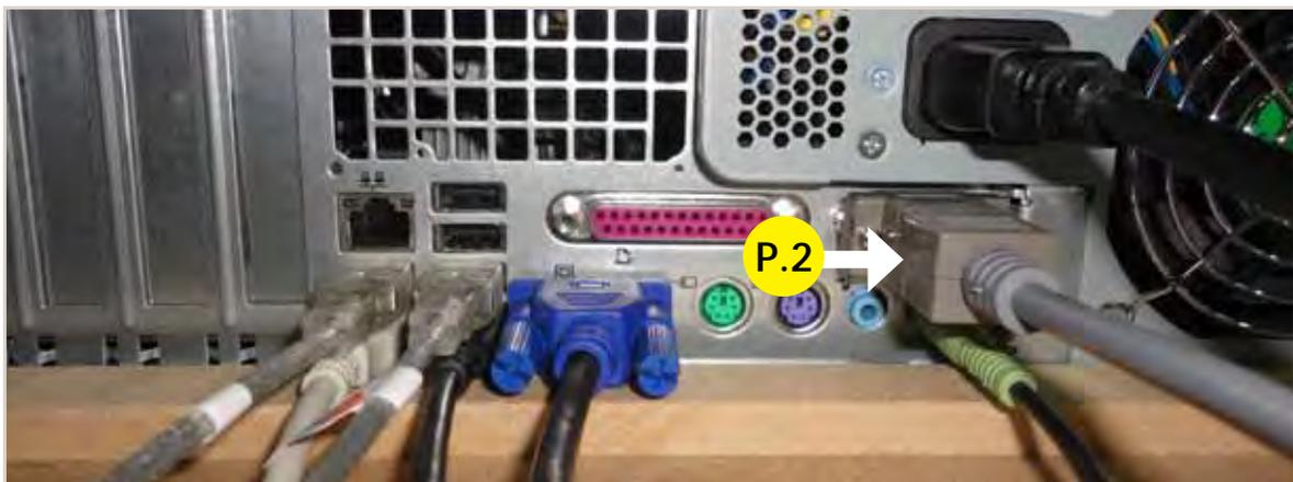
P.2 Serial Cable From to PC to Control Board. (56 cm - Inch 22,04)
