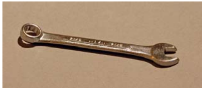
Use a 5/16 open-end / box end combination wrench on the jamb nuts.
