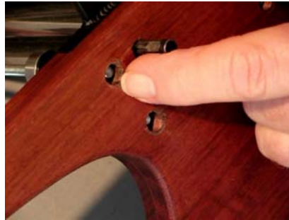
When the side piece is on, about 1/8" can be seen inside the recessed holes.
