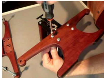
When the side piece is on, about 1/8" can be seen inside the recessed holes.
