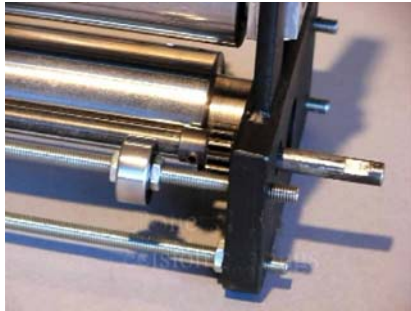
The core has four threaded cross-tie rods ends extending about 1/4".
