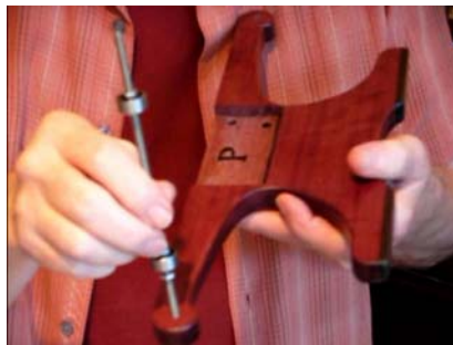
Two threaded steel cross-tie rods have a passive end, with jamb nuts and an active end
