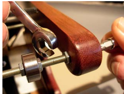
The jamb nuts in the passive side are to be snug against the wood.
