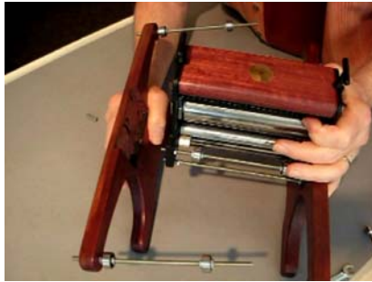
With the jamb nuts moved back, fit the side on the four threaded cross tie rods.
