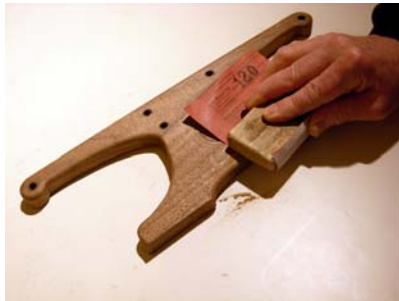
Sand before staining or oiling, start with 120 sandpaper, then steel wool to polish.
