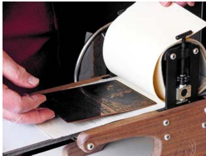
Place damp paper on the plate, settle felt blankets and turn the bed through. A slow motion turning is recommended, without stopping until you feel the roller pass of the end of the plate.
