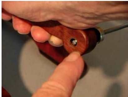
Turn the threaded cross tie rod until about 1/8" can be seen coming through, out the recessed holes. Start a barrel cap nut on this end, gripping the threaded rod so it doesn't turn with the nut.
