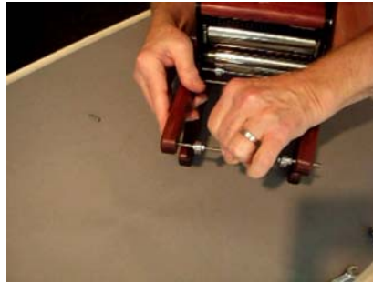
Turn the threaded cross tie rod into the threaded hole in the active side piece.
