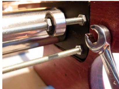
Jamb nuts inside the steel core are important to determine the 6" space where the bed travels, and so, too, the cap nut and jamb nuts on the ends of the side pieces.
