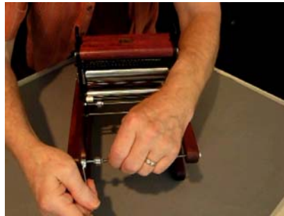
Bring the jamb nuts to the wood and secure the cap nut and jamb nut together. Measure to check for 6" bed space.
