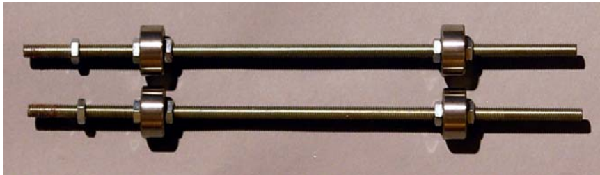
Two threaded steel cross-tie rods have a passive end, with jamb nuts and an active end
