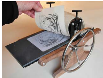
Vitreography uses either quarter-inch ground plate glass or frosted Mylar.
