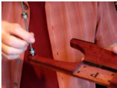
Two threaded steel cross-tie rods have a passive end, with jamb nuts and an active end
