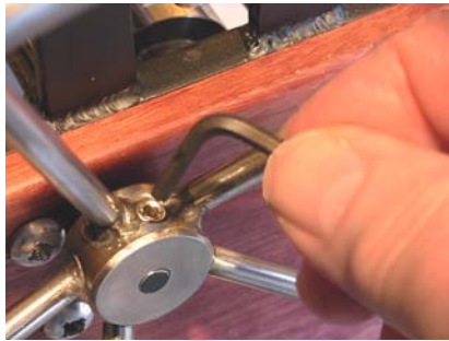
There is a fourth set screw on the wheel hub which takes the larger Allen wrench to tighten.
