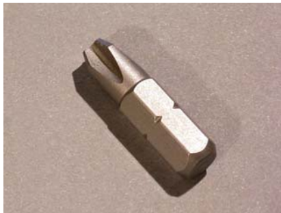
Use only the blunt-ended Philips driver bit provided for the barrel cap nuts.
