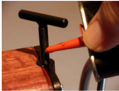
Two or three drops of light oil on the threaded pressure screws will make them turn more smoothly.
